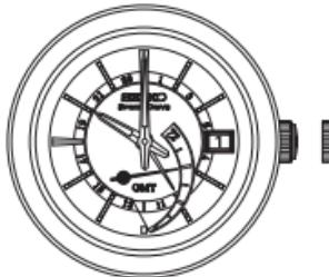
5. Turn the crown to set the hour hand to the current hour.
